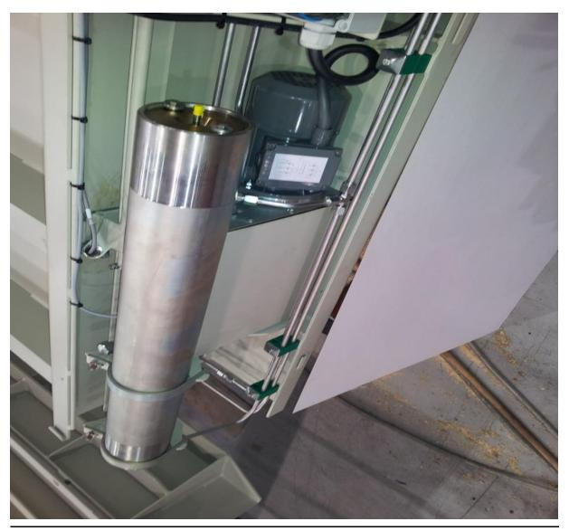
Dismount the accumulator by either open the pipe next to motor or bottom pipe under accumulator. Be careful moving the accumulator, the valve with yellow cap has a pressure of 70 bar. Dismount motor cable from junction box JB4. Under oil tank there are 3 pcs of nut, remove this.
