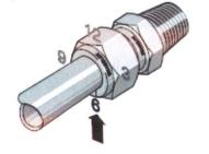
While holding the fitting body steady, tighten the nut one and one- quarter turns to the 9 o'clock position.
