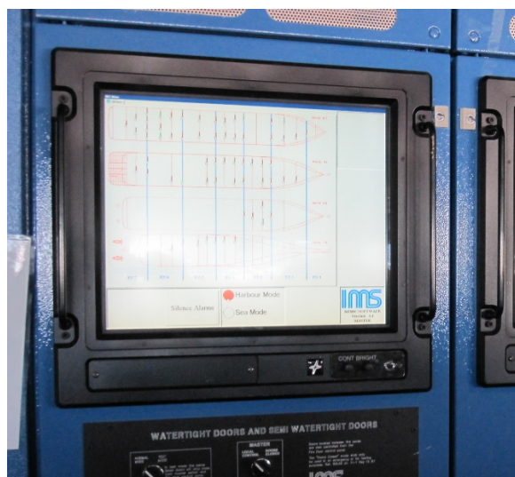
Picture 2 Typical Bridge Mimic for 2nd generation PC system
